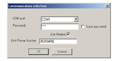
the connection to the unit; it can take up to one minute to establish the communication. When the communication will be established, the disconnect button will appear. While connected to the unit, the orange LED will turn off and no incoming calls for access control will be accepted.
